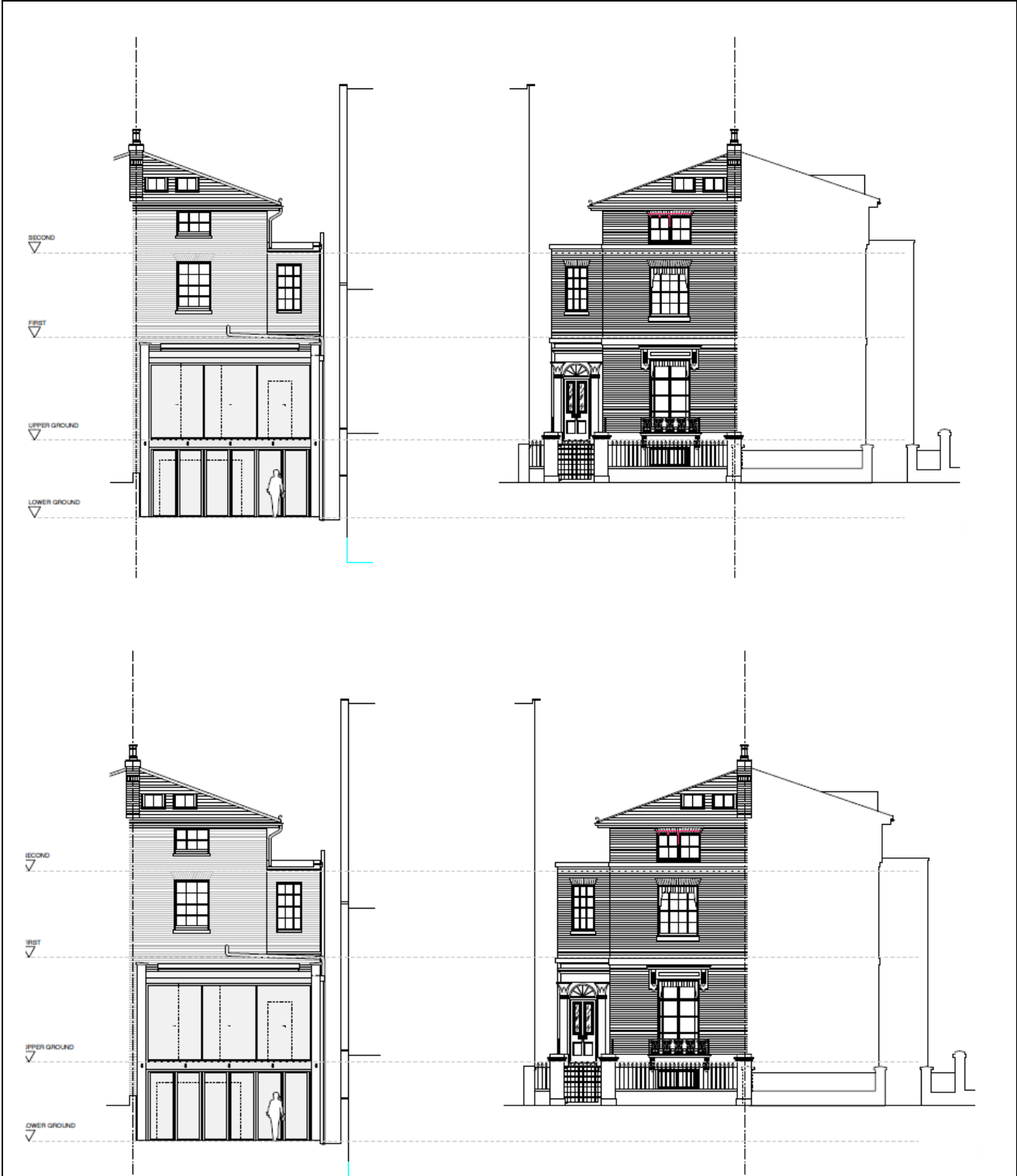
Existing front and rear elevations (top) and proposed front and rear elevations (bottom).
